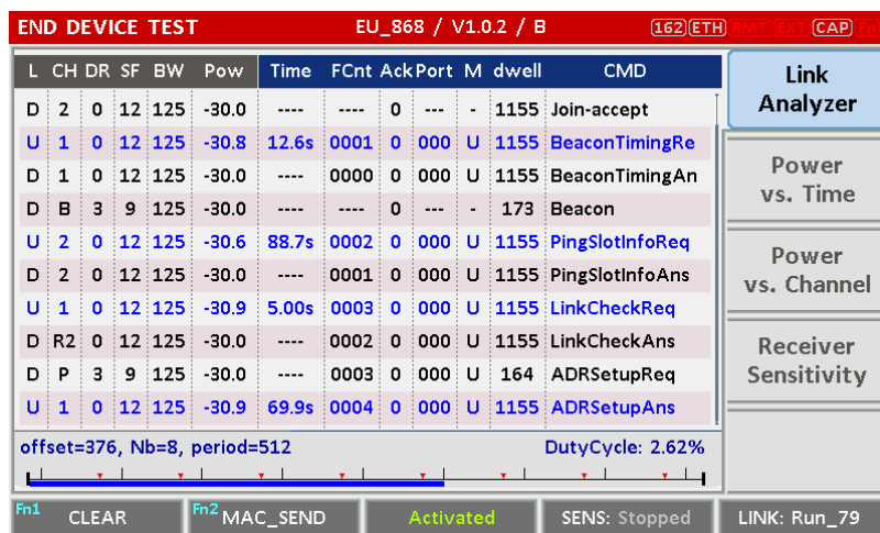
Fig 3.17 MAC command transmission through PING slot
