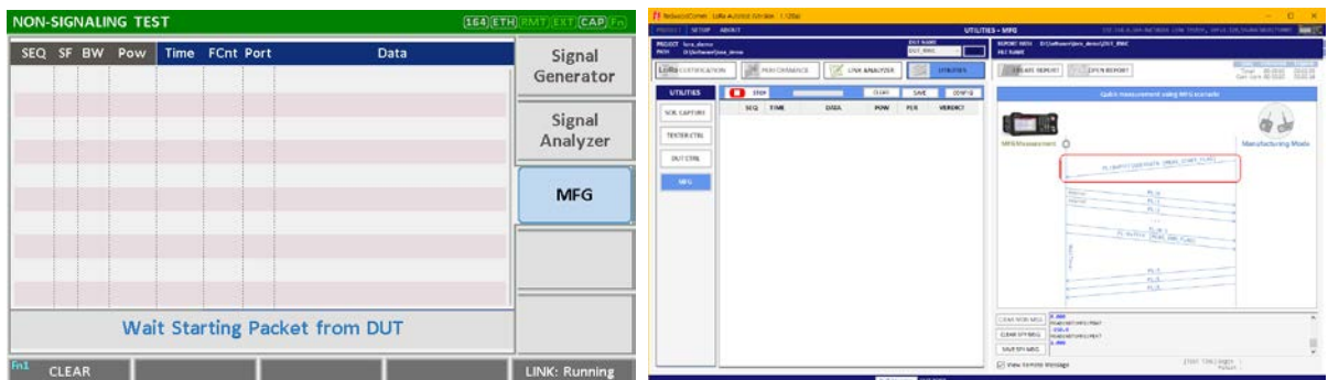
Fig 3.25 The screen of MFGA of RWC5020A and PC App. waiting for MEAS_START_FLAG from DUT
